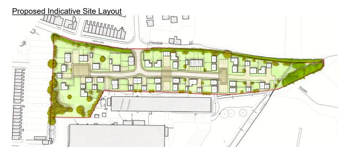
The proposal involves constructing a new access into the site from Grove Lane, forming a crossroads with Town Hill Bank. The submitted junction plan indicates that there would be a visibility splay of 2.4m by 25m in each direction along Grove Lane.
